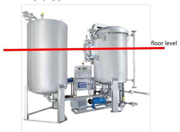
As can be seen from the above picture, a vertical package dyeing machine consists of a kier, which is a pressure vessel of sort, a carrier with spindles for holding yarn packages, inside of the kier, a pump, a piping arrangement and chemical addition system? With this said, the pump and most of the piping are located in the basement of the dye house. This, of course, adds to the capital cost of building these facilities.
