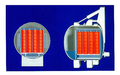
In order to minimize liquor ration, the vessel for a Horizontal Dyeing Machine should have square shape. However, high pressure inside of the vessel necessitates, in this case, a very thick vessel wall, which leads to prohibitively high cost of pressure vessel. Thus, a physical contradiction – the vessel must have round shape for high pressure reasons, and it must have square shape for supporting lower cost of operation.
